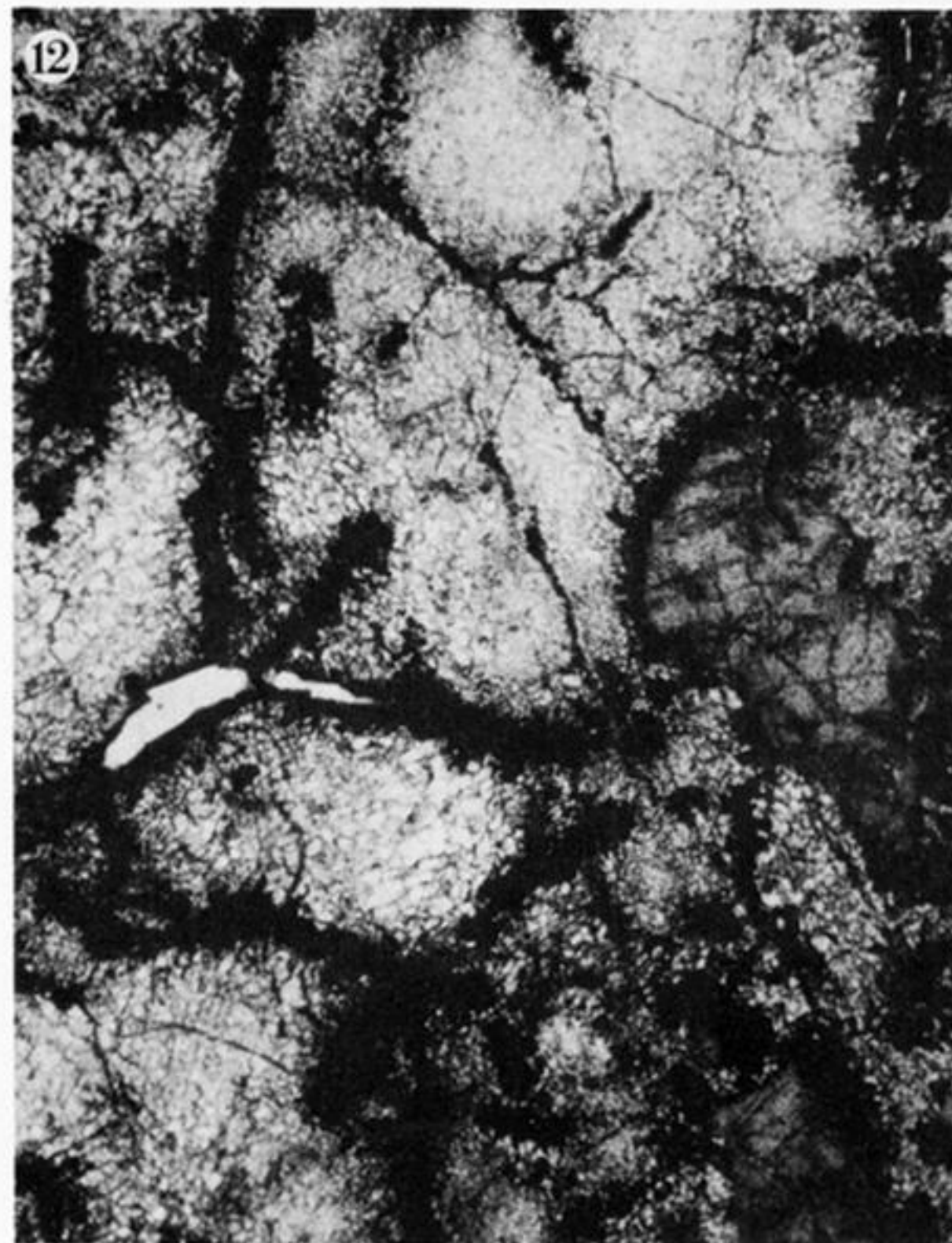
FIGURE 12. The Haverö ureilite. Large recrystallized aggregates of olivine and badly crystallized and inclusion-rich pyroxenes (dark grey) in a matrix rich in carbon (black). Some of the olivines display subparallel orientations. In the lower left corner two of such intergrowths are intergrown with each other. Note the very large elongated voids (white). Transmitted light; length of picture is 5.5 mm.
